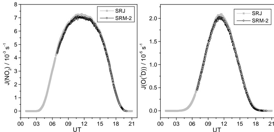
**Fig. 7.** Diurnal profiles of the photolysis frequencies  $J(\text{O}(^1\text{D}))$  and  $J(\text{NO}_2)$  measured with one collector of the SRM (SRM-2) and the SRJ on 27 May 1999 on the roof of the Institute of Atmospheric Chemistry (ICG3) (Jülich, Germany).
