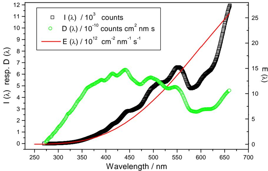
**Fig. 4.** Comparison of the irradiance  $E(\lambda)$  produced by the 1000 W-standard in a distance of 700 mm, the signal intensity  $I(\lambda)$  and the spectral response function  $D(\lambda, \theta_0)$  of one collector (SRM-3).
