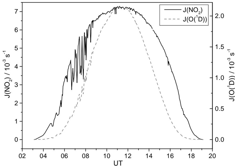
**Fig. 10.** Photolysis frequencies  $J(\text{O}(^1\text{D}))$  and  $J(\text{NO}_2)$  measured with the SRM on 9 August 1998 during the field campaign BERLIOZ in Berlin on the roof of the Charité building. Partial cloud cover in the time from 05:00 to 09:00 UT leads to reductions and enhancements in the photolysis frequencies, whereas the effect is more pronounced in  $J(\text{NO}_2)$ .
