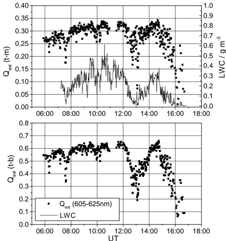
**Fig. 12.** Attenuation of the actinic flux in the cloud.  $Q_{\text{ext}}(t-m)$  is the reduction of the actinic flux from the top to the middle of tower (39 m) calculated from  $Q_{\text{ext}}(t-m) = 1 - \frac{F_{\text{B}}}{F_{\text{T}}}$ ;  $Q_{\text{ext}}(t-b)$  is the analogous reduction between the top and the bottom of the tower. The solid line in the upper panel is the liquid water content (LWC) of the cloud measured at a height of 68 m.
