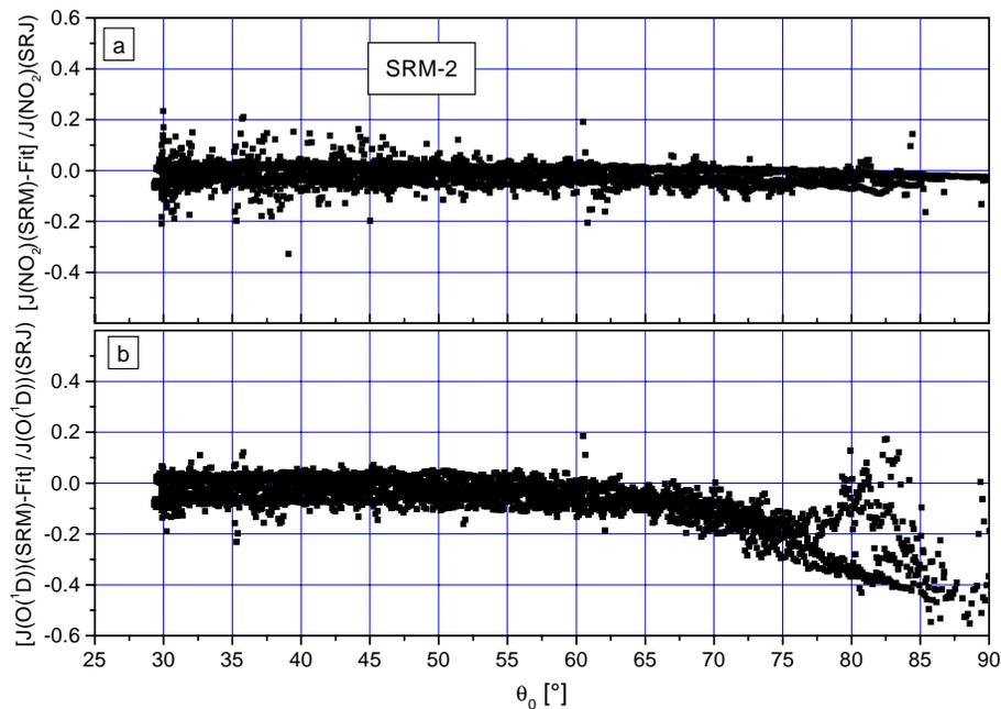
**Fig. 9.** Relative deviation of the data of (a)  $J(\text{NO}_2)$  and (b)  $J(\text{O}(^1\text{D}))$  measured with the SRM (SRM-2) from the linear best-fit lines shown in Fig. 8 as a function of solar zenith angle.
