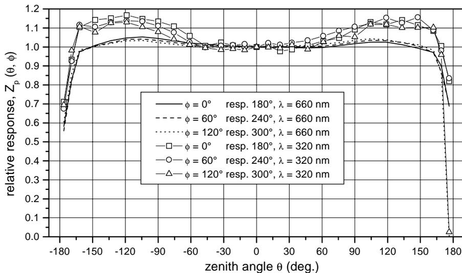
**Fig. 1.** Goniometrically determined relative response of the collector as a function of zenith angle  $\theta$  at different azimuth angles. The negative zenith angles correspond to the opposite azimuth angle, for example, the values of negative zenith angles for azimuth  $\Phi = 0^\circ$  correspond to the azimuth angle  $\Phi = 180^\circ$ .
