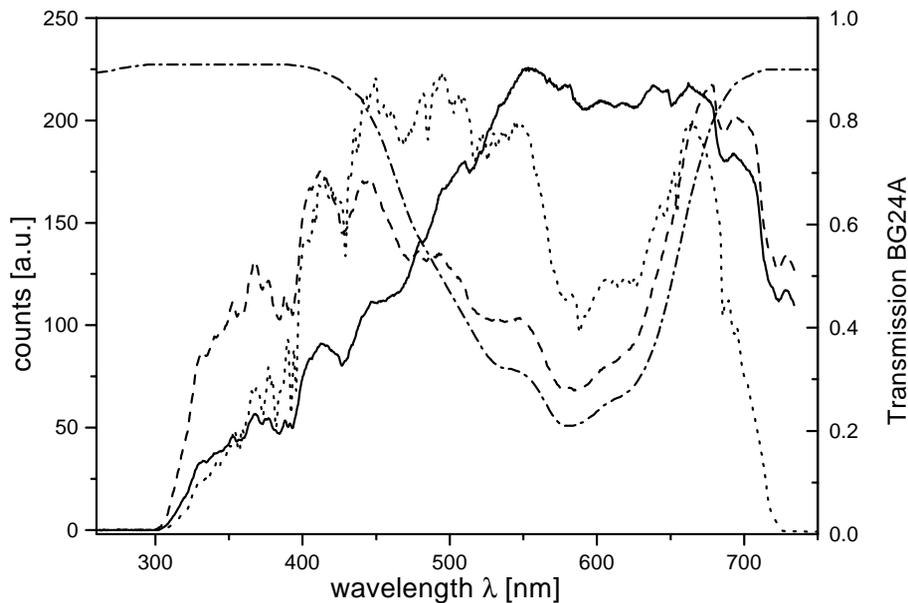
**Fig. 2.** Effects of the filter and the optical collector: (—) without either filter or optical collector, (- - -) with filter BG24A (Fa. Schott) but without optical collector; (· · · · ·) with filter BG24A, optical collector and baffle; (- · - · -) transmission of the filter. The spectra are scaled to approximately the same maximum value in the visible ranges for better illustration of the relation of the UV with equal dynamic range of the CCD.
