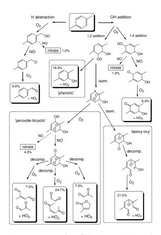
**Fig. 1.** Partial schematic representation of the OH-initiated oxidation of p-xylene to first generation products, as treated in MCM v3. The chemistry shown assumes that  $RO_2$  radicals (with the exception of that formed initially from 1,2 addition of OH and  $O_2$ ) react exclusively with NO. The first generation products are shown in boxes, and the associated percentage yields are appropriate to these conditions.
