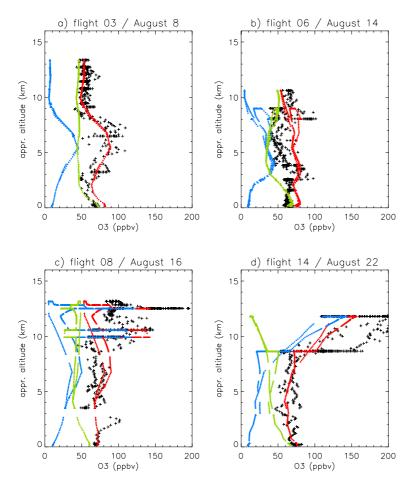
**Fig. 1.** Vertical profiles of observed ozone (black), modeled ozone (red) and contributions by O<sub>3</sub>s (blue) and O<sub>3</sub>t (green) for several MINOS flights.
