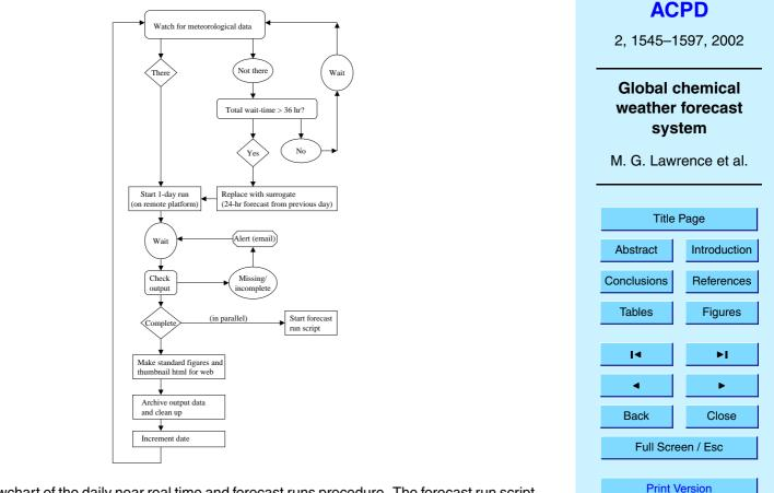
**Fig. 1.** Flowchart of the daily near real time and forecast runs procedure. The forecast run script follows the same procedure, except that no surrogates are used (the forecast run stops if the data does not become available). Within the fully-automated process there are several internal checks to ensure that the system is running as expected, with email alerts when problems arise.
