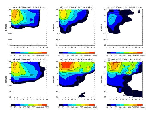
**Fig. 7.** Temporal evolution of the zonal mean Laki  $SO_4$  (pptv) for Laki Lo **(a–c)** and Laki Hi **(d–f)**, at three levels in the model: the surface (a, d); the upper troposphere (b, e); and the lower stratosphere (c, f). Background 1860 levels have been subtracted.
