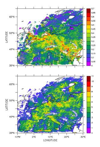
**Fig. 1.** Composite map of the **(a)** mean aerosol optical depth at  $0.555 \, \mu \text{m}$  over Europe for August 1997 and **(b)** the number of observations used to derive the mean value. AOD has been retrieved by application of the dual view algorithm to the ATSR-2 satellite data over land and the single view algorithm over ocean.
