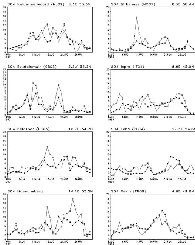
**Fig. 3.** Daily variation of modelled (filled squares) and measured (empty squares) sulphate and (total) nitrate concentrations in  $\mu\text{g}/\text{m}^3$  at selected locations in Europe. Data obtained from EMEP (2002) ([www.emep.int](http://www.emep.int)) and Zimmerling et al. (2000).
