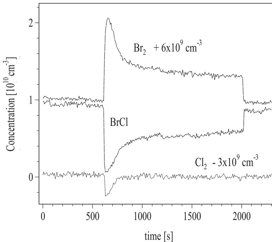
**Fig. 7.** Uptake of  $\text{BrCl}$  and  $\text{Cl}_2$  onto a mixed, frozen salt surface and formation of  $\text{Br}_2$ .  $T = 233 \text{ K}$ ,  $2 \text{ M NaCl}$ ,  $3 \times 10^{-3} \text{ M NaBr}$ . The  $\text{Br}_2$  and  $\text{Cl}_2$  traces have been offset for clarity of presentation.
