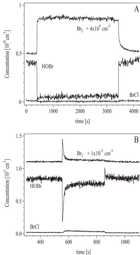
**Fig. 3.** Uptake of HOBr and subsequent product formation, on a frozen mixed salt surface at 233 K. **(a)**  $[\text{HOBr}]_{\text{init}} = 4 \times 10^9$  molecules  $\text{cm}^{-3}$ , exposure of the surface to HOBr begins at 400 s when the injector is retracted. **(b)**  $[\text{HOBr}]_{\text{init}} = 8.5 \times 10^{10}$  molecules  $\text{cm}^{-3}$ , exposure of the surface to HOBr begins at 550 s. In both cases, the  $\text{Br}_2$  trace has been offset for clarity of presentation.
