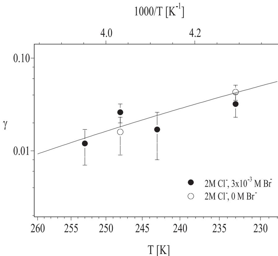
**Fig. 6.** Temperature dependence of the initial uptake coefficient of HOBr onto frozen surfaces made from solutions containing 2 M NaCl with and without added NaBr. The error bars define the reproducibility of the result.
