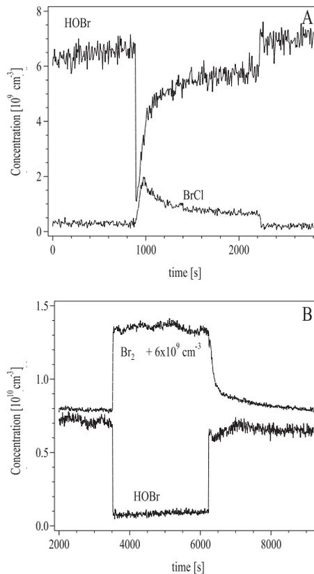
**Fig. 5.** Uptake of HOBr onto frozen salt surfaces. **(a)** 2 M NaCl,  $T = 233 \text{ K}$ , **(b)**  $3 \times 10^{-3} \text{ M}$  NaBr, 243 K. The  $\text{Br}_2$  trace has been offset for clarity of presentation.
