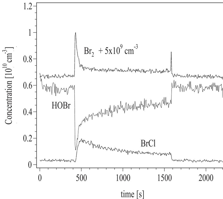
**Fig. 4.** Uptake of HOBr onto a frozen (233K) mixed salt surfaces made from an aqueous solution of composition 2 M NaCl,  $3 \times 10^{-4}$  NaBr. The  $\text{Br}_2$  trace has been offset for clarity of presentation.
