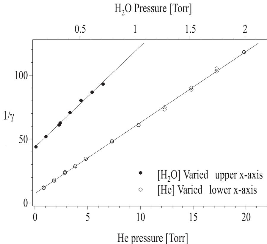
**Fig. 2.** Plot of inverse uptake coefficient of HOBr vs. pressure of He or  $\text{H}_2\text{O}$ , for dry salt and HCl doped Pyrex surfaces at 253 K. Diffusion coefficients and accommodation coefficients may be extracted from the gradients and intercepts of these lines. (See Eq. iii in text)
