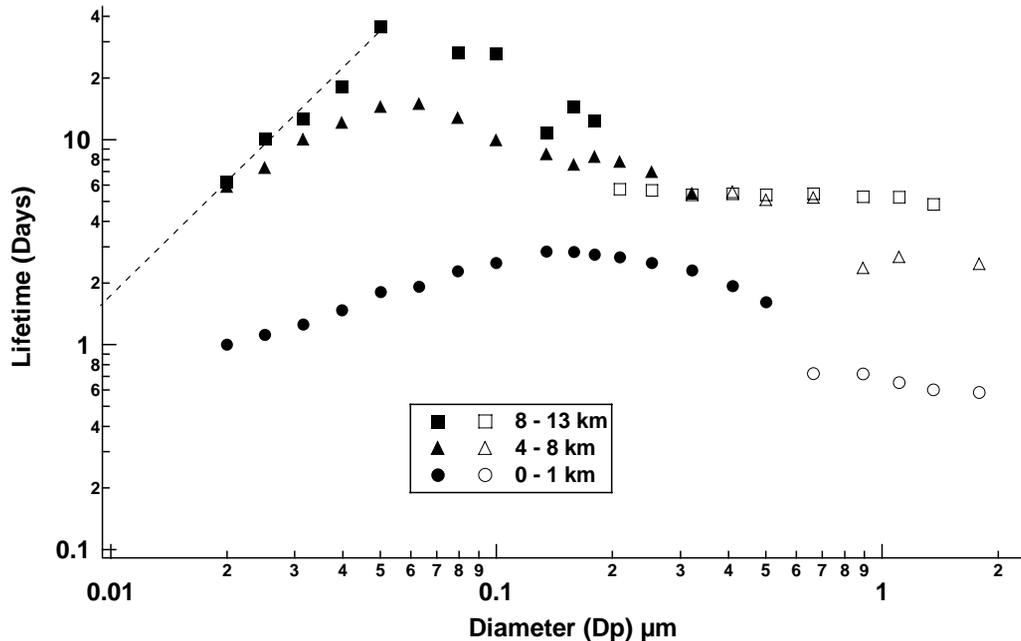
**Fig. 5.** Lifetime of particles as a function of size for the INDOEX region in February 1999, estimated by fixing the lifetime of the 20 nm particles to the modelled coagulation lifetime. Filled symbols indicate that the “in situ”  $b$  coefficient was used whereas open symbols indicate that the “injected” coefficients were employed. The dashed line shows the extrapolation to 10 nm particle lifetimes for comparison with Schröder et al. (2000).
