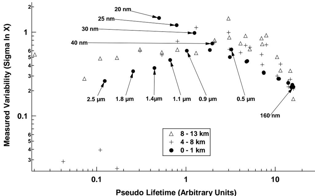
**Fig. 4.** Measured variability plotted against arbitrary lifetime derived from an adapted version of the Jaenicke expression. Solid circles represent data from 0–1 km, crosses represent data from 4–8 km, and triangles show data from 8–13 km.
