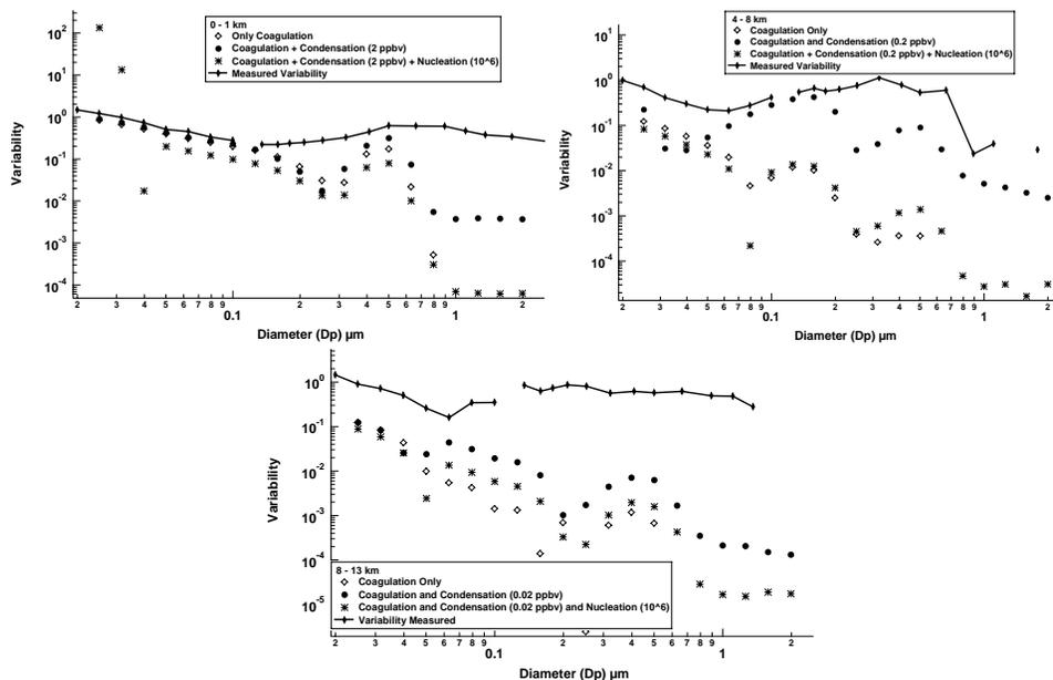
**Fig. 3.** Comparison of measured variability and of variability predicted by the model for coagulation, coagulation and condensation and coagulation, condensation and nucleation, between (a) 8–13 km, (b) 4–8 km, (c) 0–1 km in February of the INDOEX campaign intensive field phase.
