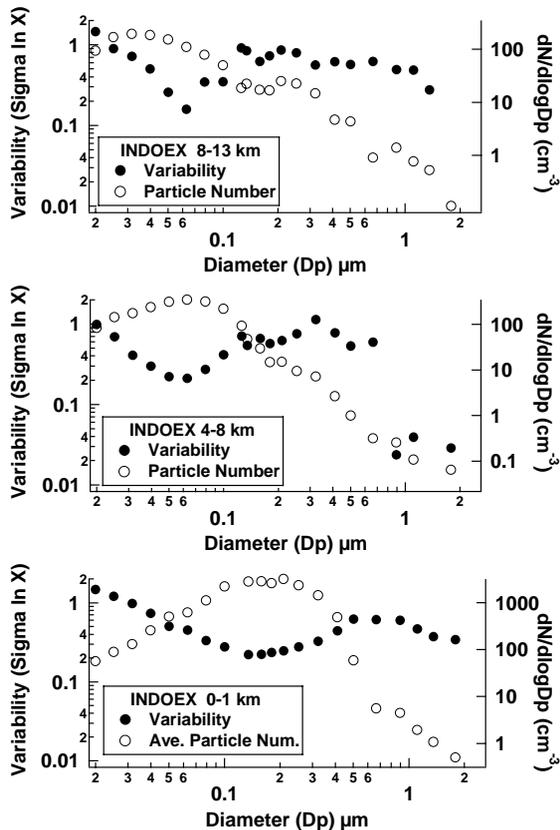
**Fig. 2.** Measurement variability and average number concentration are plotted as a function of bin size for data collected between (a) 8–13 km, (b) 4–8 km, (c) 0–1 km in February of the INDOEX campaign intensive field phase.
