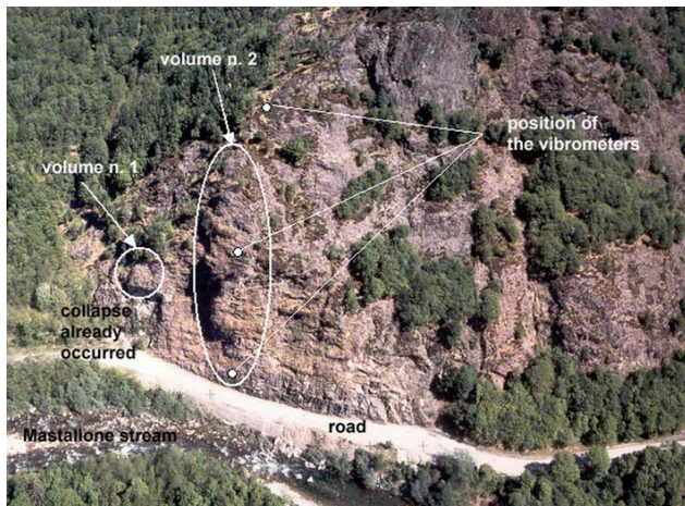
Fig. 2. Panoramic view of the unstable rock slope on the Mastallone valley (North of Italy).
