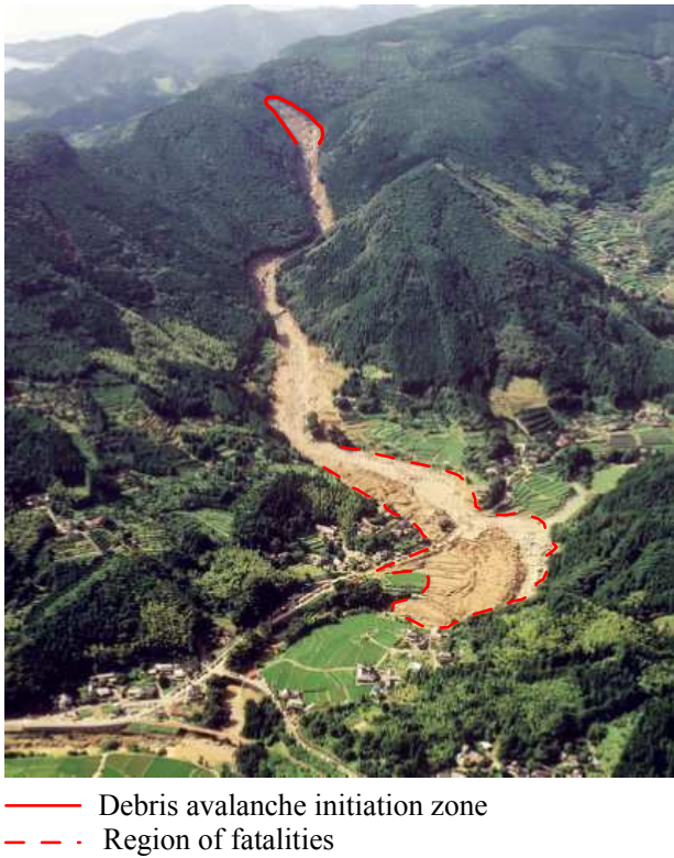
Fig. 4. Aerial photograph of destroyed village and the path of the debris flow.
