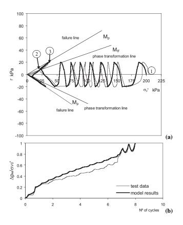
**Fig. 2.** Cyclic shear stress test on loose saturated undrained sand: experimental data vs. constitutive model numerical results. (a) Stress path, failure and phase transformation lines. (b) Liquefaction degree  $(\Delta p_w/\sigma'_{v0})$  (after Wijewickreme et al., 2005).
