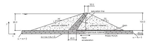
Fig. 4. Geometry of the studied earth dams. Saturation line, types of material and boundary conditions.
