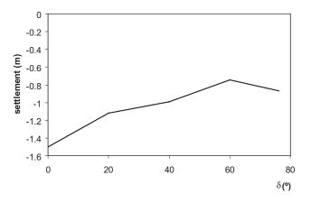
Fig. 12. Settlement of the crest dam at the end of the Vancouver horizontal accelerogram, against the angle of the impervious core,  $\delta$ .
