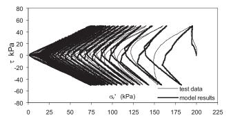
**Fig. 3.** Cyclic shear stress test on dense saturated undrained sand. Stress path: experimental data vs. constitutive model numerical results (after Wijewickreme et al., 2005).
