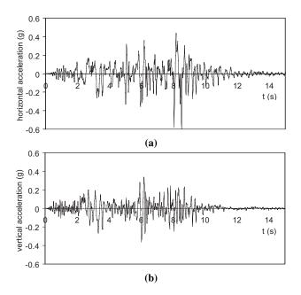
**Fig. 5.** Recording at the Pacoima dam (CDMG Station 279), San Fernando earthquake (9 February 1971), scaled to a maximum horizontal acceleration,  $|a_{hmax}| = 0.6$  g. (a) Horizonal accelerogram (254). (b) Vertical accelerogram. (http://nisee.berkeley.edu/).
