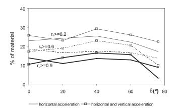
**Fig. 8.** Percentage of dam material over the depicted liquefaction degrees,  $r_u$ , against the angle of the impervious core,  $\delta$ , at the end of the San Fernando earthquake. Results for only horizontal and both horizontal and vertical accelerations are provided.
