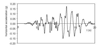
**Fig. 10.** Horizonal accelerogram reported by Byrne (2005), which has a 2% probability of being exceeded in 50 y in the Vancouver area.
