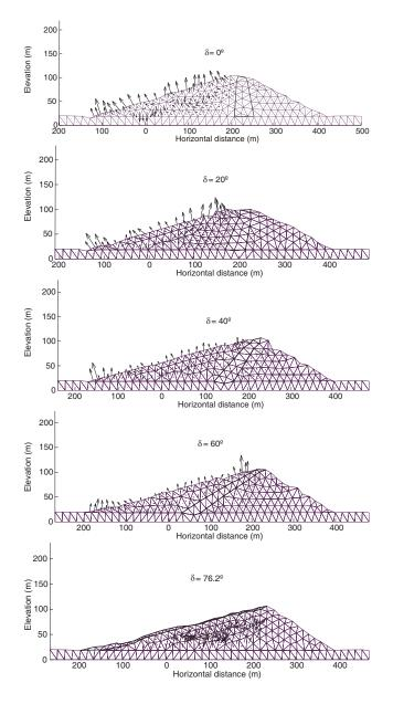
**Fig. 7.** Deformed shapes (amplification factor = 50) of the analysed dams at time t=8.52 s of the San Fernando earthquake (subjected only to its horizontal component). The vectors show the directions of the water flow inside the dams.
