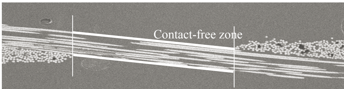
Figure 4. Transverse cut of a coated glass plain weave, contact free zone
