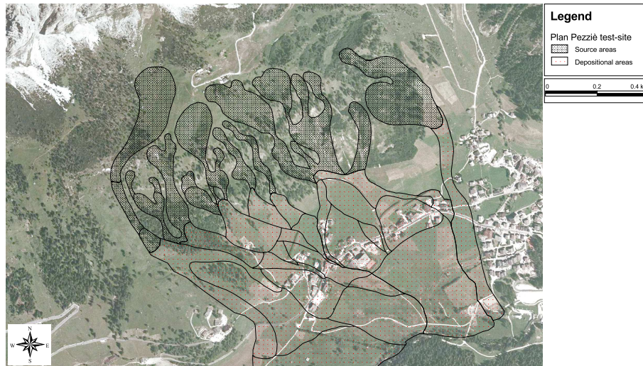
Fig. 4. Plan Pezziè test-site. Source and depositional areas of earth-debris flows are represented. Debris cones are mapped as indicators of high landsliding activity over long periods (royalties on Digital Orthophoto: Autonomous Province of Bolzano-Autonomie Provinz Bozen-Sudtiro).
