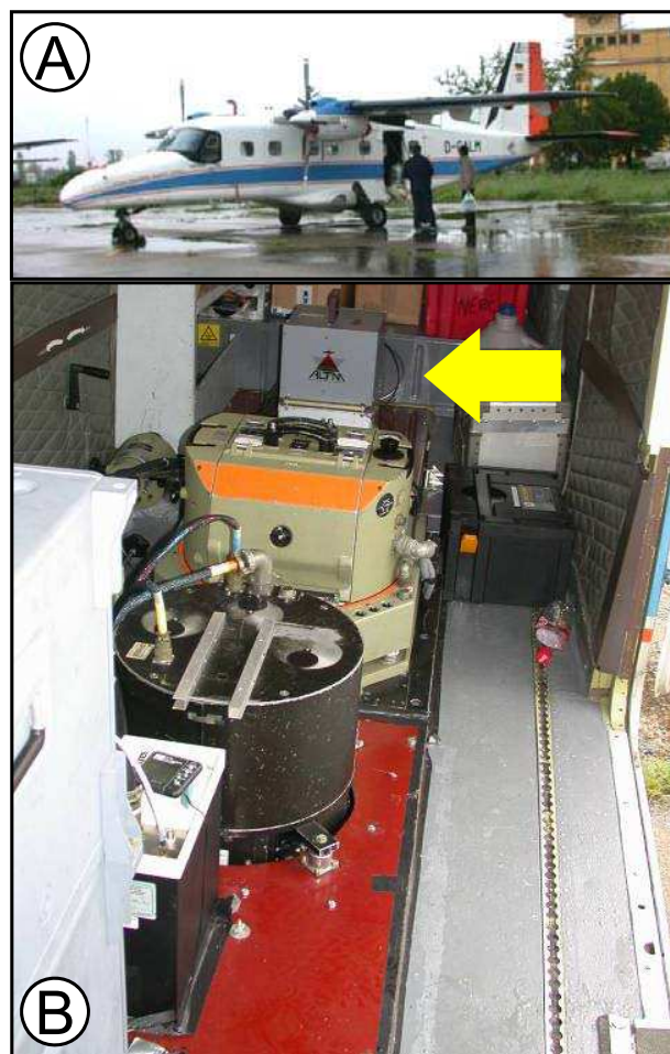
Fig. 6. (A) Dornier 228-110 aircraft operated by the Airborne Research and Survey Facility of the UK National Environment Research Council that flew the Optech's Airborne Laser Terrain Mapper 3033, shown by the arrow in (B).
