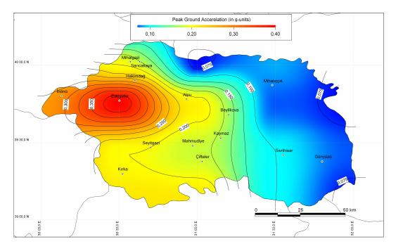
Fig. 5. Seismic hazard from all source zones for rock site based on Gülkan and Kalkan (2002) attenuation relationship (475-year return period).
