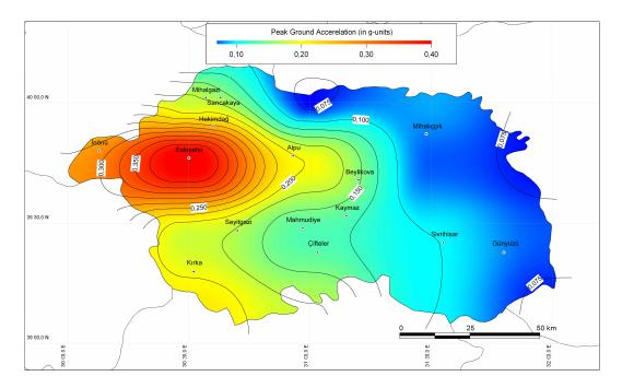
Fig. 4. Seismic hazard from all source zones for rock site based on Boore et al. (1997) attenuation relationship (475-year return period).
