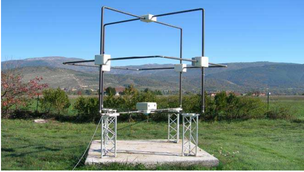
Fig. 1. Three axes induction antenna for magnetic field measurement in the frequency band [1Hz–100 kHz]. The instrumental sensitivity is equal to 1 fT / \sqrt{Hz} .
