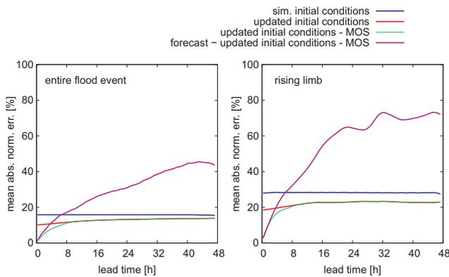
**Fig. 3.** Average forecast errors  $e_j$  of the five flood events of Table 2. Entire flood event (left), rising limb only (right). Kamp at Zwettl, 622 km<sup>2</sup>.
