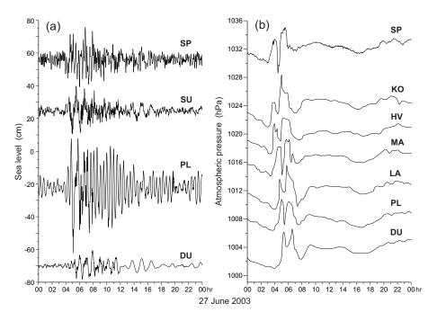
**Fig. 14.** (a) The high-frequency component of the sea level time series for Split, Sućuraj, Ploče and Dubrovnik. Low-frequency oscillations have been removed by a high-pass digital filter with a cut-off period of 2 h. (b) High-resolution air pressure oscillations measured at a number of microbarographs during the meteotsunami event of 27 June 2003.
