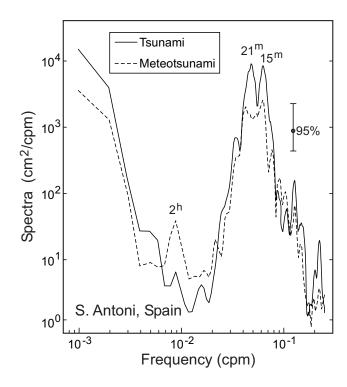
**Fig. 6.** Sea level spectra for the tsunami of 21 May 2003 and the moderate meteotsunami event of 1 May 2003 recorded at Sant Antoni (Ibiza Island, Spain). Each event has a duration of 4 days with a sampling interval of 2 min (2880 points). Spectra have been estimated with a Kaiser-Bessel window (cf. Emery and Thomson, 2001) of 128 points with half-window overlaps resulting in 42 degrees of freedom.
