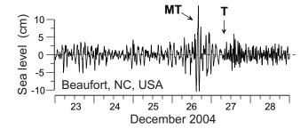
**Fig. 2.** Sea level oscillations at Beaufort (North Carolina, USA) for the period 23–28 December 2004. "MT" indicates intensive seiche oscillations generated by a strong storm travelling northward along the east coast of North America; "T" marks the arrival time of tsunami waves associated with the 2004 Sumatra earthquake (Rabinovich et al., 2006).
