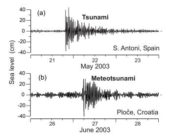
**Fig. 1.** (a) Tsunami oscillations recorded at Sant Antoni (Ibiza Island, Spain) after the Algerian earthquake of 21 May 2003; and (b) the meteotsunami recorded at Ploče Harbour (Croatia) on 27 June 2003. Both records have been high-pass filtered to eliminate oscillations with periods longer than 2 h.
