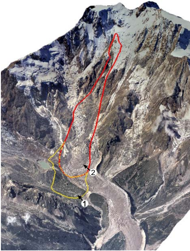
Fig. 3. Transition zone and deposit area of the ice/rock avalanche in August 2005. The reach of the solid part of the avalanche (rock and ice) is marked in red; the reach of the powder avalanche is marked in yellow. No. 1 indicates the location of the hut Zamboni, no. 2 points to the location of the Lake Effimero, which is not visible on this aerial photograph from 1999.
