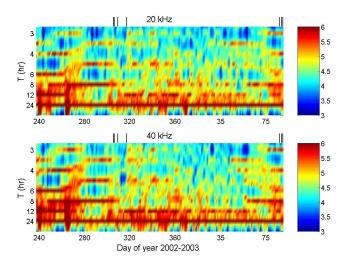
**Fig. 9.** Dynamic spectrum in logarithmic scale of the 20 kHz and 40 kHz VLF signals for the time period September 2002–March 2003. The lines in the upper border indicate the occurrence time of earthquakes (Md > = 4). Colour bars indicate the power density in (pT)<sup>2</sup>/Hz.
