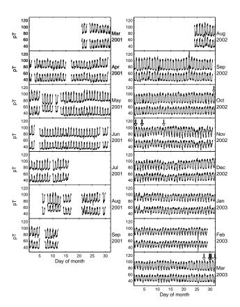
**Fig. 6.** VLF data (1 min averages) for the time periods March–September 2001 and September 2002–March 2003. The arrows indicate the occurrence time of earthquakes (Md > = 4). Upper curves show 40 kHz data (upward shifted by 20 pT), lower curves show 20 kHz data.
