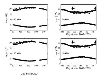
Fig. 8. Morning and afternoon terminator time for March–September 2001 (left) and September 2002–March 2003 (right). The arrows indicate the occurrence time of earthquakes (Md > = 4).
