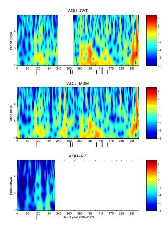
**Fig. 5.** Dynamic spectrum in logarithmic scale of the daily differences AQU-CVT, AQU-MDM and AQU-RIT for the years 2002–2003. Black curves indicate the "cone of influence", where edge effect becomes important. The lines in the lower border indicate the occurrence time of earthquakes (Md > = 4). Colour bars indicate the power density in  $(nT)^2/Hz$ .
