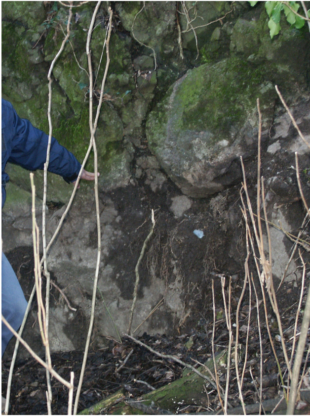
Fig. 5. Vertical offset between stable basaltic cliff and dismembered blocks.
