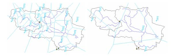
Fig. 6. Raingauges networks and Thiessen polygons on the Savinja catchment.
