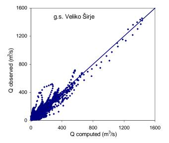
Fig. 4. Comparison of computed and observed discharges for the period 1998–1999.
