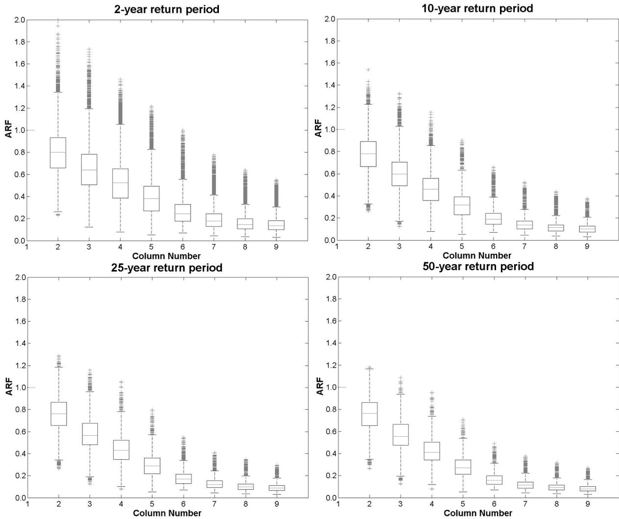
Fig. 5. Box plots of the data sample for each return period selected and the 120-min duration.
