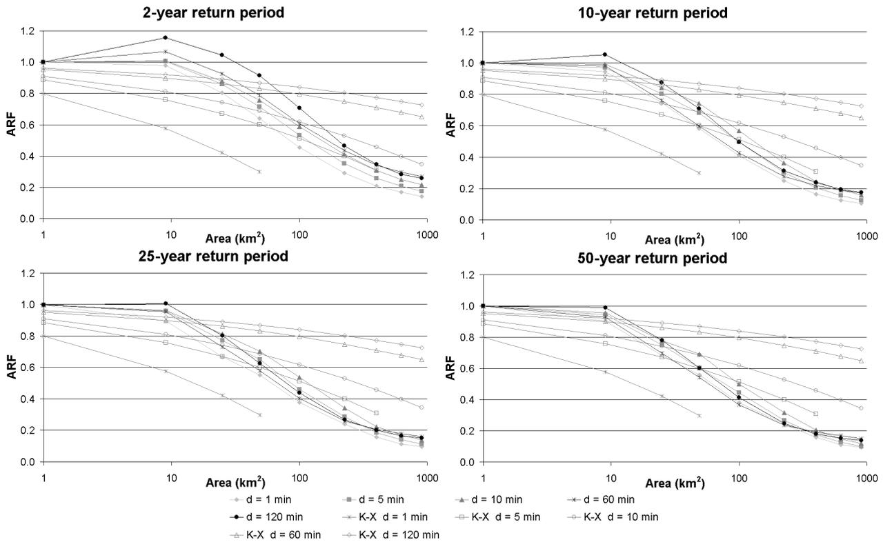
**Fig. 8.** Semi-logarithmic plots of the ARF trends with increasing area for various durations and return periods shown against ARF-area Koutsoyiannis and Xanthopoulos relationship which is a function of the area and the duration.
