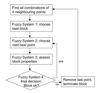
Fig. 7. General scheme of the block detection algorithm.
