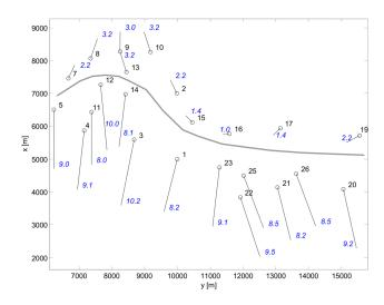
**Fig. 8.** Graphical representation of the displacement vectors of the example given. The length of the vectors (in mm) is given in italic at the end point of the vectors. The grey curve is showing the boundary between the stable and the unstable areas.
