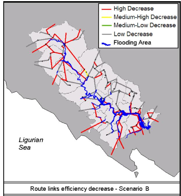
**Fig. 8.** Representation of the road network of the Vara basin, in which each road link is characterized on the basis of the difference between its physical integrity and the efficiency obtained in connection to Scenario B. The flood area relevant to this scenario (namely, the flood area characterized by T=500 years) is represented in blue.
