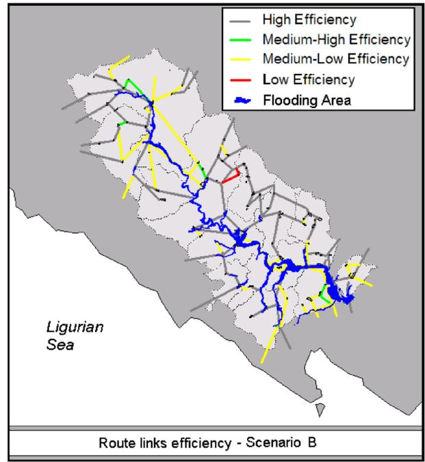
**Fig. 7.** Representation of the road network of the Vara basin, in which each road link is characterized on the basis of the efficiency obtained in connection to Scenario B. The flood area relevant to this scenario (namely, the flood area characterized by T=500 years) is represented in blue.
