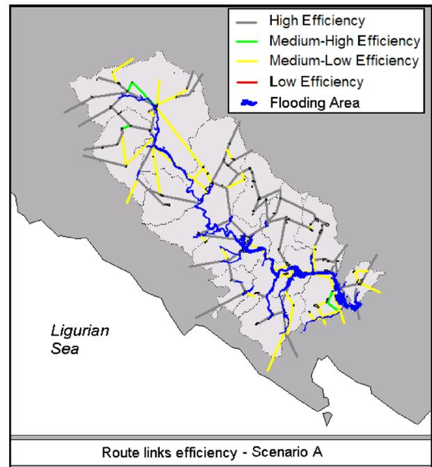
**Fig. 4.** Representation of the road network of the Vara basin, in which each road link is characterized on the basis of the efficiency obtained in connection to Scenario A. The flood area relevant to this scenario (namely, the flood area characterized by  $T=200$  years) is represented in blue.
