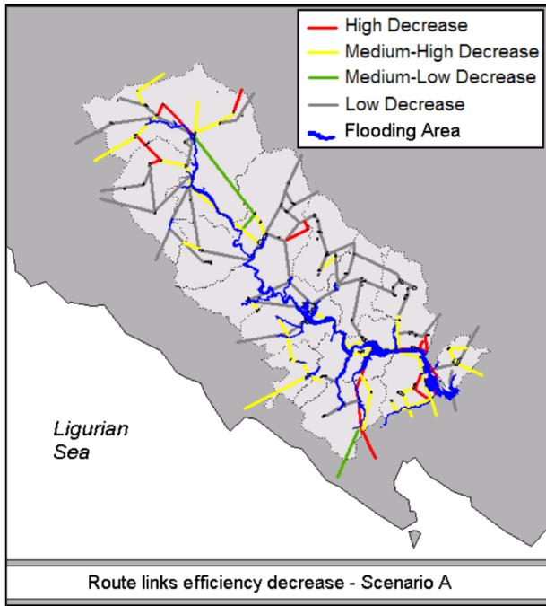
**Fig. 5.** Representation of the road network of the Vara basin, in which each road link is characterized on the basis of the difference between its physical integrity and the efficiency obtained in connection to Scenario A. The flood area relevant to this scenario (namely, the flood area characterized by T=200 years) is represented in blue.
