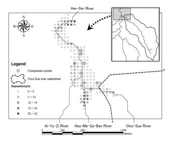
Fig. 5. Results of the numerical simulation.
