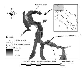
**Fig. 4.** Distributions of average thickness of deposition and erosion along Chui-Sue River from micro-geomorphic study.
