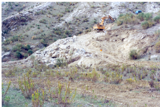
Fig. 10. Gypsum and alabaster mining areas near the village of Mëngaj (Kavaje district). Messinian evaporites have been the object of intensive extraction, without considering the presence of several karst caves, some of which have been destroyed by the mining activity. Protests from environmentalists and scientists eventually resulted in stopping the activities, thus saving at least a karst cave located few tens of meters apart from where the caterpillar is (north-western corner of the photo).
