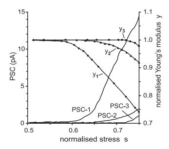
**Fig. 5.** Variations of the recorded PSCs (solid lines) and the corresponding Young modulus *y* with respect to the normalized stress, during the three loading processes.
