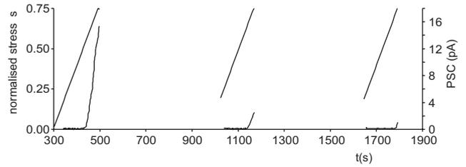
**Fig. 2.** PSCs recordings during the three sequential loading cycles in the range of the normalized stress,  $0 < s < 0.75$ .
