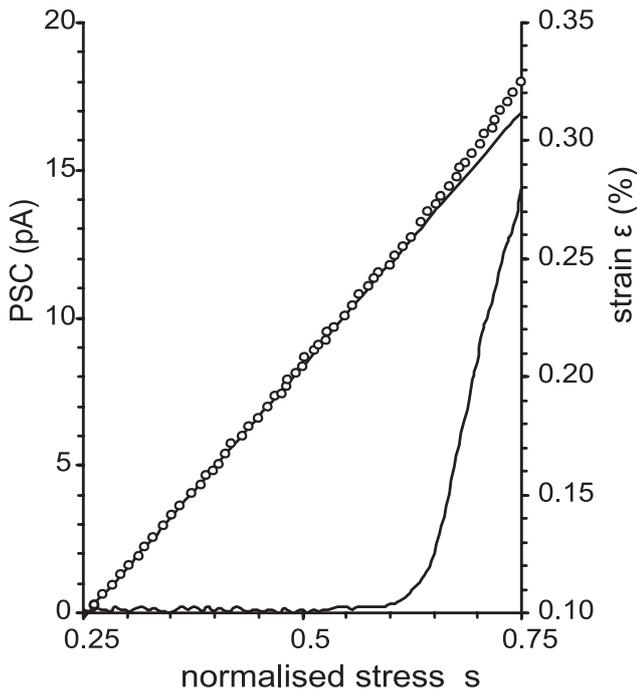
**Fig. 3.** PSC-1 recordings as a function of normalized stress,  $s$ . The stress – strain variation for  $s$  values up to 0.75 is also shown. The dotted line represents the extension of the linear (elastic) region.
