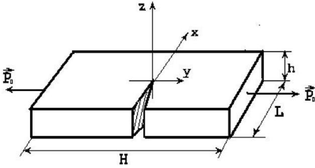
**Fig. 1.** The crack for the simple case of quartz, the optical axis is oriented in the  $Z$  direction and the magnetic moment caused by circular vortical polarization current in the plane of the crack is oriented along the same axis. Here  $P_0$  is the mechanical stress (Makarets, 2002).
