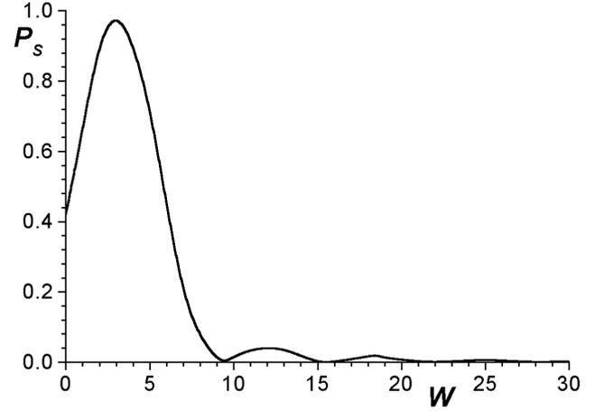
**Fig. 2.** The dependence of the power of seismo-electromagnetic wave  $P_S$  (relative units, connected with the ratio of the radiation energy to the mechanical energy  $P_S = \frac{P_e}{P_m}$ ) caused by the single crack in the quartz on the undimensional frequency  $w = \omega \frac{L}{v}$ .
