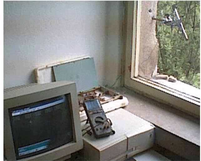
Fig. 2. The magnetometer with sensor and PC.
