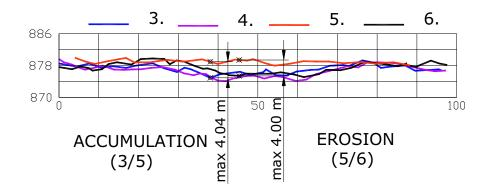
Fig. 10. A comparison for the reference cross section "ST\_KOS1 - CD2" for the measurement sets in 2004.
