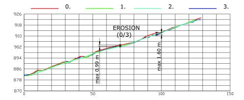
Fig. 7. A comparison of the reference cross section "ST\_KOS1–ST\_KOS2" for the measurement sets in 2003.
