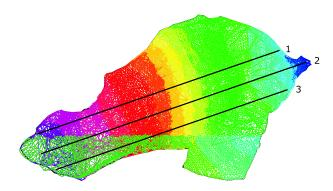
**Fig. 11a.** 3-D TIN model of the Strug rock fall area derived from the aerial photographs taken on 28 December 2001, just after the initiation of the rock fall. Position of the three selected longitudinal profiles for their time evolution comparison are also given.
