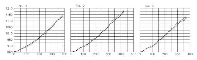
Fig. 12. Three longitudinal profiles of the Strug rock fall – comparison between 3-D TIN models of December 2001 (thin lines) and September 2003 (thick lines).
