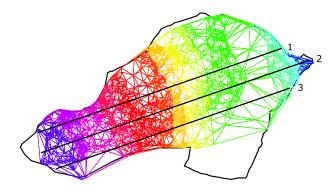
**Fig. 11b.** 3-D TIN model of the Strug rock fall source area derived from geodetic measurements in September 2003 using laser scanner measurement system. Position of the three selected longitudinal profiles for their time evolution comparison are also given.
