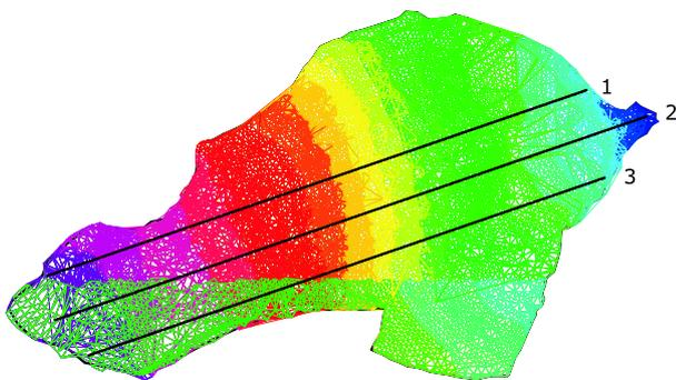
**Fig. 11a.** 3-D TIN model of the Strug rock fall area derived from the aerial photographs taken on 28 December 2001, just after the initiation of the rock fall. Position of the three selected longitudinal profiles for their time evolution comparison are also given.
