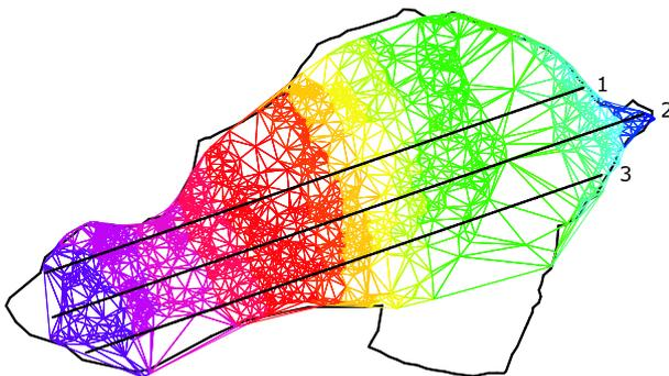
**Fig. 11b.** 3-D TIN model of the Strug rock fall source area derived from geodetic measurements in September 2003 using laser scanner measurement system. Position of the three selected longitudinal profiles for their time evolution comparison are also given.
