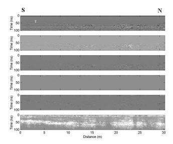
**Fig. 4.** Processing step performed on the radar data acquired with 500 MHz antenna: (a) raw radar section; (b) background removal filter; (c) Kirchhoff migration; (d) gain function removal; (e) amplitude compensation; (f) envelopes. The reflections (labelled T) are produced by the top of the cave.
