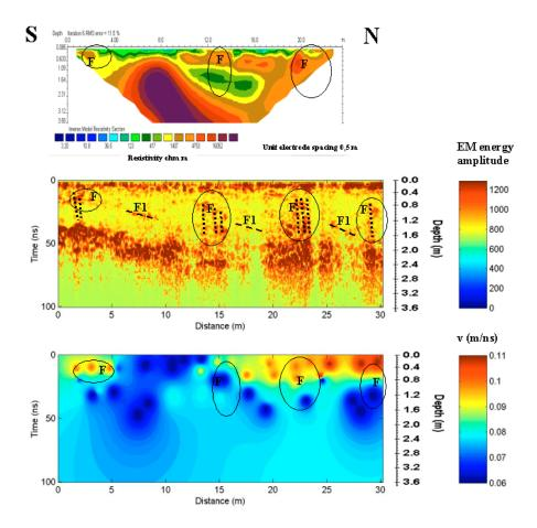
**Fig. 5.** Survey results: **(a)** 2-D electrical resistivity model; **(b)** envelopes processed radar section: the fracture with high EM energy scattering are labelled F and F1; **(c)** EM wave velocity variation model. The integrated geophysical analyses outlined a highly unstable region in the investigated area.
