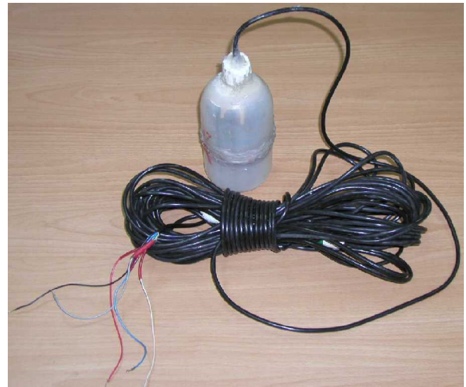
Fig. 3. Sealed GD crustal stress transducer and the cable.
