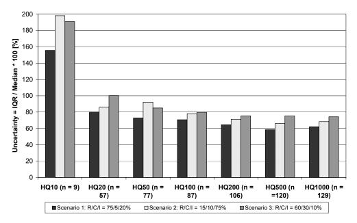
Fig. 8. Influence of building use composition on the uncertainty of flood damage estimates for different return periods. Considered economic sectors: private housing, services sector and manufacturing.
