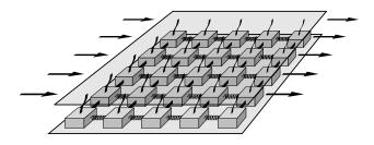
**Fig. 5.** Setup of a two-dimensional spring-block model. Blocks are connected with each other and with a rigid driver plate through springs and leaf springs, respectively.
