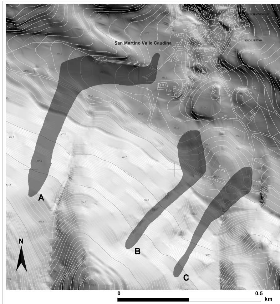
Fig. 4. The Vallicelle (San Martino V. C.) debris flows of December 1999: from left to right, the cases of study A-C utilised in the calibration phase of SCIDDICA S_3\text{-hex} (after PAI-Hydrogeological setting plan, in press).
