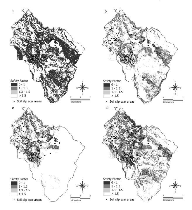
**Fig. 7.** Slope stability maps from the simulation with different hydrological models: (**a**) steady state model (SSM); (**b**) piston flow model with uniform precipitation (PFM\_UNI); (**c**) piston flow model with distributed precipitation (PFM\_DIS); (**d**) diffusive model with distributed precipitation (DM\_DIS). Results for the diffusive model (DM\_DIS) are relative to the maximum soil thickness. Areas with different computed safety factors are reported.
