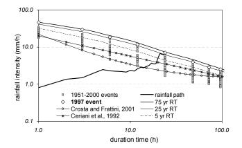
**Fig. 6.** Recurrence time of rainfall events at Bellano rain gauge compared with the 27–28 June 1997 maximum intensities and rainfall pattern (defined as cumulative rainfall normalized by rainfall duration). Two rainfall thresholds for shallow landslide triggering in Alpine areas are reported (Ceriani et al., 1992; Crosta and Frattini, 2001).
