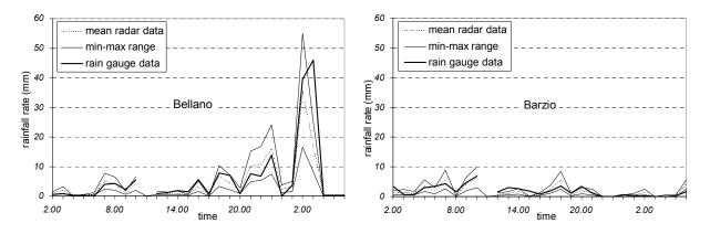
**Fig. 3.** Hourly rainfall data from 02:00 LT of 27 June to 06:00 LT of 28 June 1997 from Bellano and Barzio rain gauges. Radar data at 30 min time interval, from Mount Lema station (Swiss Meteorological Institute), have been hourly averaged for comparison with rain gauge data.
