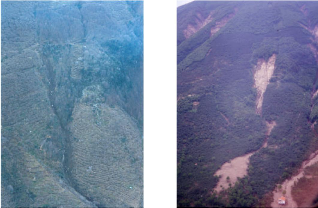
**Fig. 10.** Comparison from 1997 to 1998 of the main landslides in Lagno Cisierno: the photo at left was taken by A. Santo (University of Naples) on 24 January 1997, few days after the 1997 event; photo at right was taken in June 1998, about one month after the May tragic event. Note the different extent of the area affected by landsliding, and in particular the enlargement of the main landslide area toward the west (to the right in the photos).
