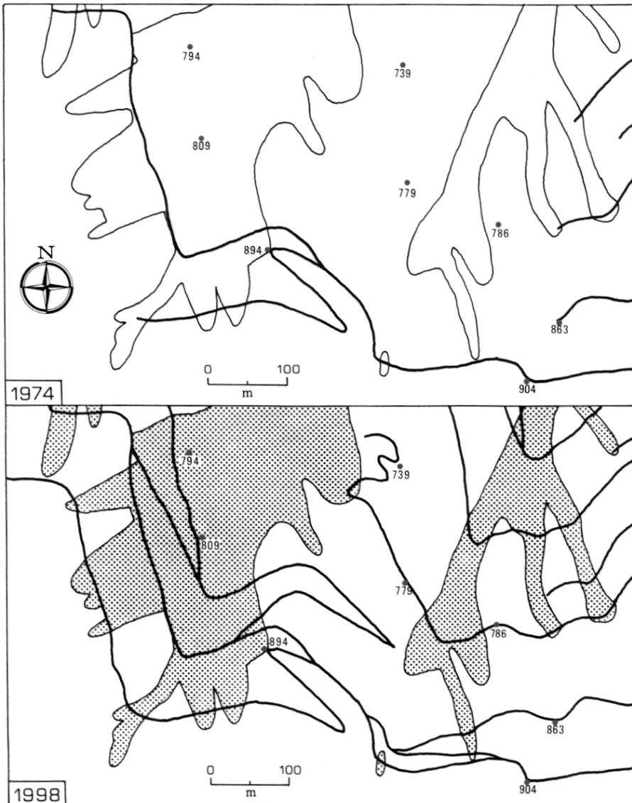
**Fig. 9.** Maps showing evolution of the pathways (boldlines) from 1974 to 1998 in the Connola – S. Francesco area. Note the high increase of pathways in the considered time span, and the proximity of many 1998 landslide source areas to the pathways. Moreover, it has to be mentioned that interpretation of the 1968 set of air-photos showed that at that time no pathway was present in the same area.
