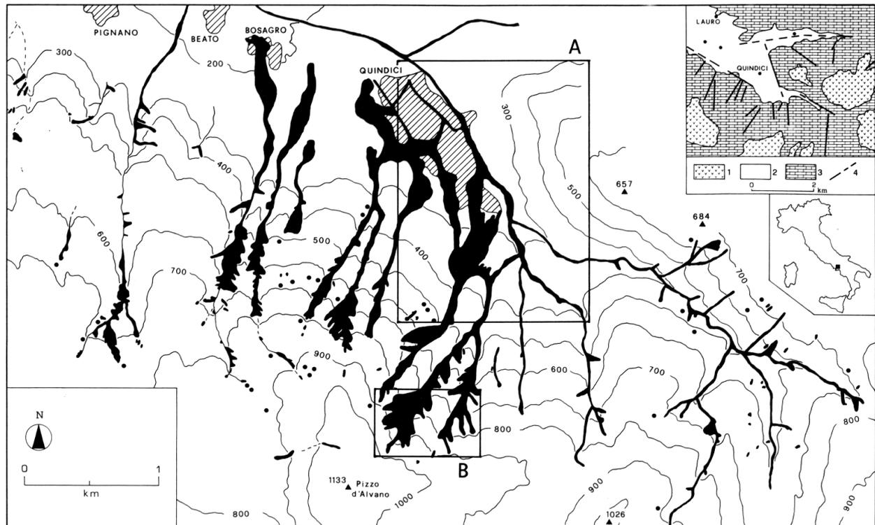
**Fig. 1.** Distribution of the 5 May 1998 landslides in the Quindici area. Small dots indicate the location of unmappable slope failures. Rectangle A refers to Fig. 5, rectangle B to Fig. 9. Contour interval 100 m. In the inset, geological sketch of study area. Legend: (1) Pyroclastics (Holocene – Late Quaternary); (2) Alluvial and fan deposits (Holocene – Quaternary); (3) Carbonate bedrock (Tertiary – Mesozoic), mantled by pyroclastics and epiclastics; (4) Fault (presumed when dashed).
