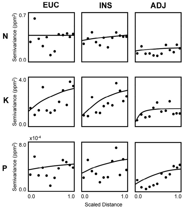
**Fig. 3.** Semivariograms for nutrient concentrations N, K, and P in the stream (rows) fitted with exponential models developed using Euclidean (EUC), symmetric in-stream (INS), and adjusted (ADJ) distance metrics (columns).
