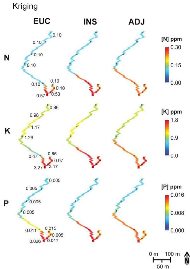
**Fig. 4.** Example of the ordinary kriging interpolations for nutrient concentrations N, K, and P (rows) using Euclidean (EUC), symmetric in-stream (INS), and adjusted (ADJ) distance metrics (columns). The circles in the figure show the locations and concentrations of nutrient observations. The location of this example relative to the entire watershed is indicated in Fig. 2.
