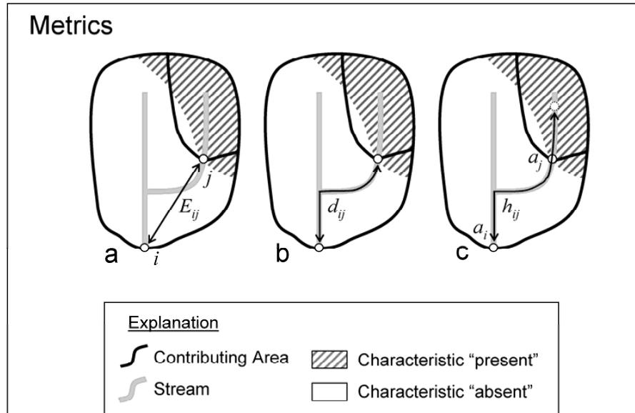
**Fig. 1.** Schematic watershed showing the difference between (a) Euclidean, (b) symmetric in-stream, and (c) adjusted distance metric for two points  $i$  and  $j$ . For the adjusted distance metric, the two points virtually move further apart because the spatial distribution of the selected landscape characteristic is very different for the two local contributing areas.
