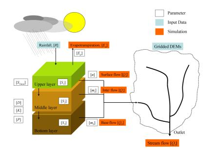
Fig. 2. Schematic diagram of the 3-layer TOPMODEL.
