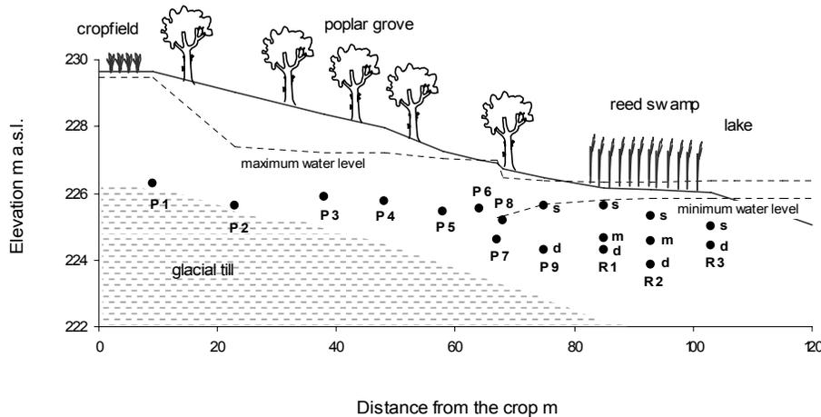
**Fig. 2.** Vertical cross section of the experimental field. The maximum and minimum recorded water levels are shown. Codes represent piezometer nest locations. • = indicate position of the piezometers screen.
