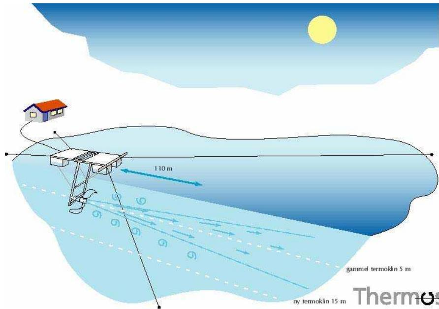
**Fig. 3.** Schematic sketch of the propeller used to deepen the thermocline in Lake Breisjön.
