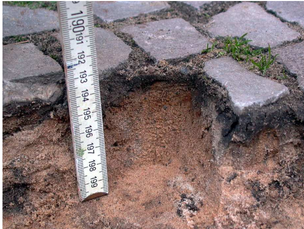
Fig. 2. Dark seam material (0 to 1 cm) compared to the lighter original sandy seam filling (1 to 5 cm) at Weidendamm, Berlin.
