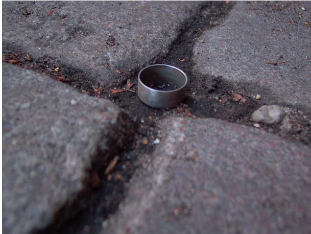
Fig. 4. Undisturbed sampling of seam material (0 to 1 cm) from a cobbled stone paved street using special 3.3\text{ cm}^3 cylinders in an old residential area at the site Pfluegerstrasse, Berlin.
