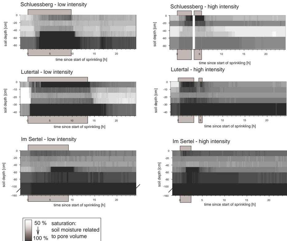
**Fig. 6.** Soil moisture dynamics at different sites in response to different precipitation intensities. Values of soil moisture are given in relation to pore volume, which was estimated according to Sponagel et al. (2005) from grain size distribution and packing density. Grey shaded boxes indicate sprinkling periods.
