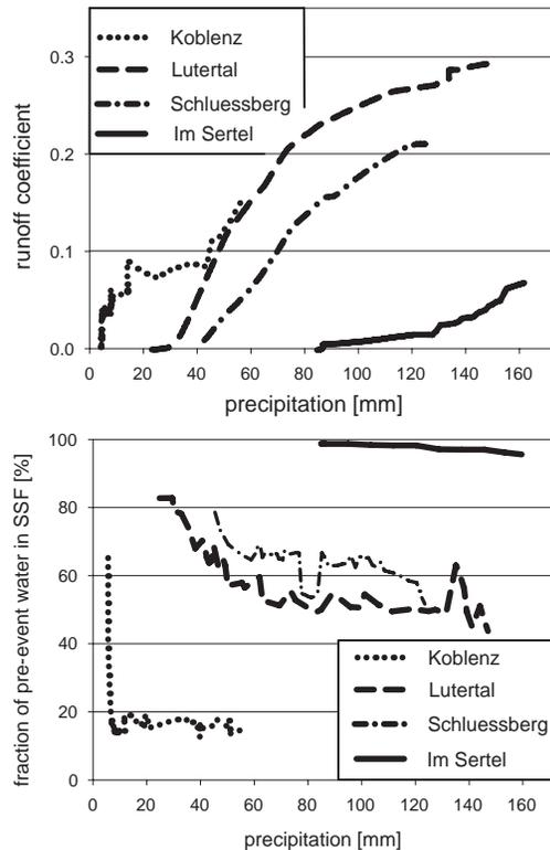
**Fig. 2.** Intercomparison of differently responding hillslopes (Kienzler and Naef, 2007). Directly fed subsurface storm flow starts quickly and contains little pre-event water (Koblenz). Indirectly fed subsurface storm flow starts delayed and consists mainly of pre-event water (Im Sertel). Experimental slopes Lutertal and Schluessberg responded in between these extremes. Results of pre-event water fraction and cumulative runoff coefficient are plotted against cumulated precipitation sum.
