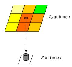
**Fig. 2.** The traditional  $Z_e$ –R matching method (TMM).
