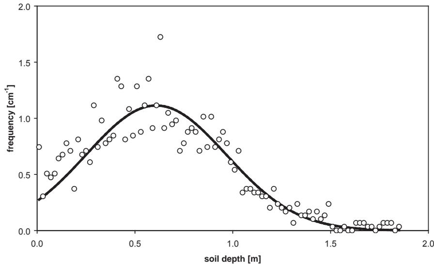
**Fig. 8.** Soil depth distribution at Panola (Georgia, USA). The measured distribution of soil depth was fitted with a normal distribution function. The mean of the fitted distribution is 0.609 m with a standard deviation of 0.358 m. The coefficient of variation was used for the storage capacity distribution function as well.
