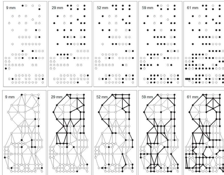
**Fig. 1.** Patterns of transient saturation as a function of rainstorm amount measured at Panola (Georgia, USA). Locations of piezometers with a water table during the rainstorm event are shown with black disks; dry sites are shown with open circles. In the bottom row, a grid connecting the sites is shown for visualization purposes. Thick lines connect two sites with free water. For 59 and 61 mm of rainstorm amount, a network of connections between open sites spans the whole system.
