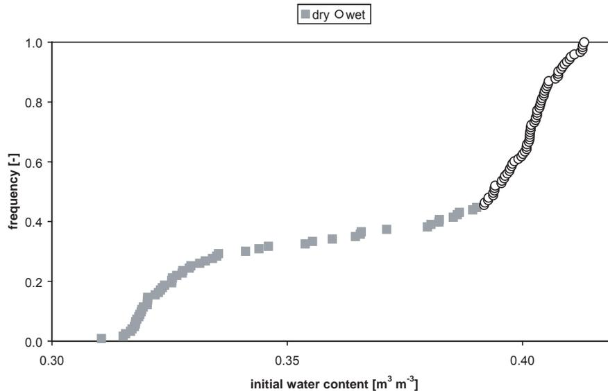
**Fig. 7.** Initial water content at Panola (Georgia, USA). The distribution of the initial water content before the rainstorm events measured at 70 cm. Two classes of initial water content are defined. The threshold value between the “dry” (grey squares) and the “wet” (open circles) condition was chosen as  $0.391 \text{ m}^3 \text{ m}^{-3}$ .
