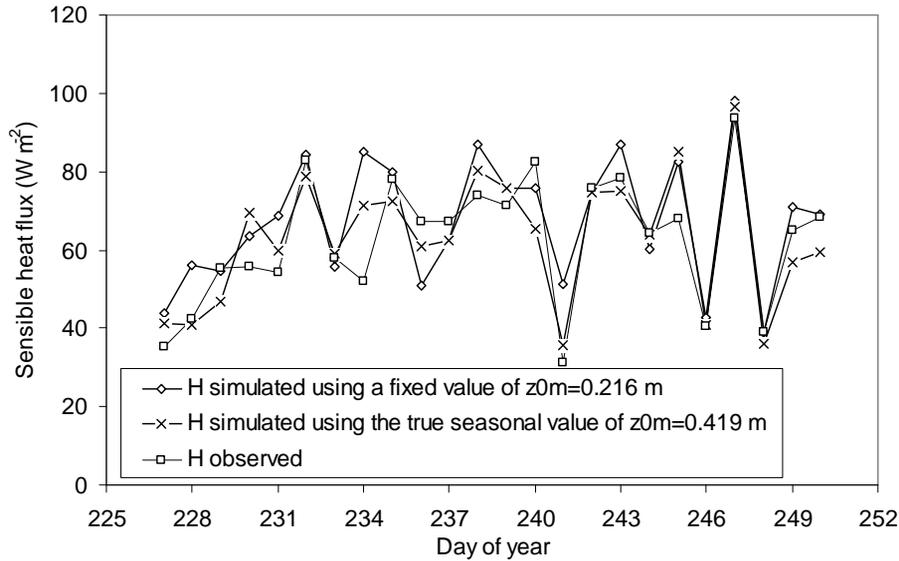
Fig. 4. Comparison between the observed and simulated sensible heat flux from DOY348 to DOY365.
