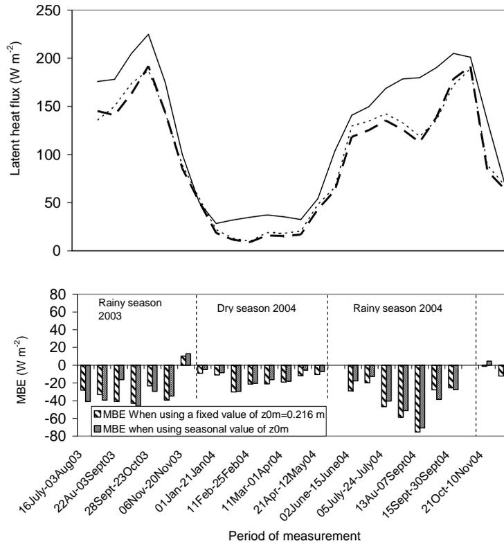
**Fig. 1.** Comparison between the observed and simulated latent heat flux on a seasonal basis. The solid line corresponds to the measured latent flux, the bold dashed line corresponds to the simulated latent heat using a fixed value of  $z_{0m}$ , while the light dashed line corresponds to the simulated latent heat flux using the seasonal values of  $z_{0m}$ .
