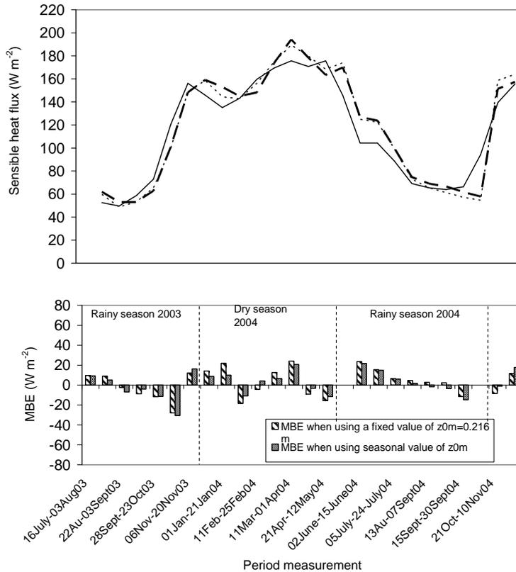
**Fig. 2.** Comparison between observed and simulated sensible heat flux on a seasonal basis. The solid line corresponds to the measured sensible heat flux, the bold dashed line corresponds to the simulated sensible heat using a fixed value of  $z_{0m}$ , while the light dashed line corresponds to the simulated sensible heat flux using the seasonal values of  $z_{0m}$ .
